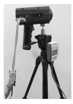
Your scoreboard package includes a radar gun kit. The radar gun can capture the speed of pitches and relay that information to your control console, which sends the data to be displayed on your scoreboard. The radar gun is battery operated and therefore does not require AC power during the game (as long as you keep the battery charged). It communicates wirelessly with the scoreboard control console, so there are no additional cables to run.
