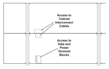
the back of the scoreboard, this access panel will be just to the right of the left-hand post. Above this access panel, at the top of the lower cabinet, is the panel covering the lower set of interconnect cabling. Just above this, in the top cabinet, is the panel covering the upper set of interconnect cabling.
